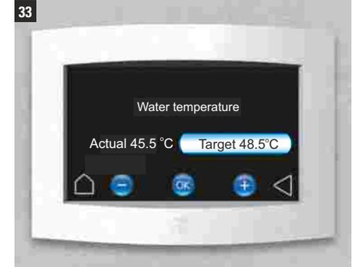
Press the **Target** icon to highlight and then press **+** or **-** icons to increase or decrease the target temperature. Confirm with **OK**.
