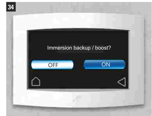
**INFO** Your HPW 300 is fitted with an electric immersion heater as a backup (or to boost heating capacity to reduce reheating times). The standard 1.5kW immersion will half the reheat time.
