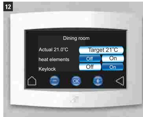
Touch the **Target** icon to set your required temperature in the respective room using + or -.
