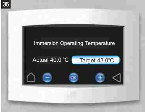
Press the **Target** icon to set your required temperature using + or - icons. Confirm with **OK**.
