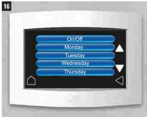
Touch the **24/7 Programmer** icon to access the configuration menu of your customised time program. This allows you to define varying ventilation levels for different times of the day. For example, you may want to set **Level 1** (background ventilation) for periods of the day when the house is unoccupied and **Level 2** as a default for when the house is occupied.
