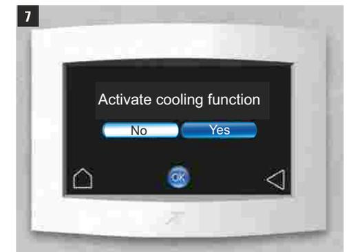
You can only activate the **cooling function** to provide active cooling in **Comfort Mode** and **ECO Summer** operating modes. The effect is to also reduce the relative humidity level.
