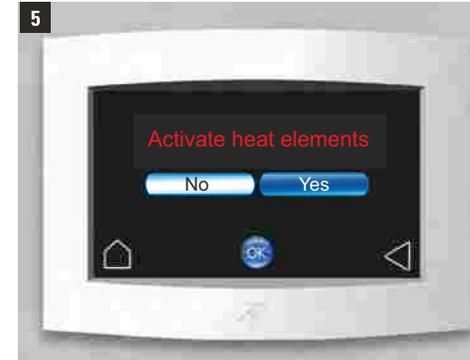
The heating elements are the ancillary terminal heaters and/or inline duct heaters. Heating elements can only be enabled in **Stove Mode**, **Comfort Mode** and **ECO Winter** operating modes.
