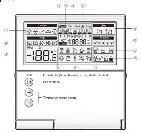
• Without opening the cover of your wired remote controller, you can turn CONTROL KIT on or off or set the desired temperature.
